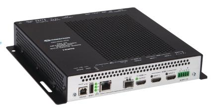
secure web-based control and management, auto-switching HDMI® inputs and output, analog audio in or out, USB 2.0 and KVM integration, video wall processing, native Dante® or AES67 transmit and receive capability, and support for copper and fiber LAN connectivity, the DM-NVX-352 offers a one-stop solution for any-sized network AV installation. [2,3]
