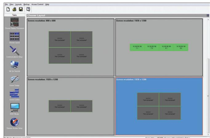
The control software is organized into a series of tasks shown on the left, designed so that the user can easily navigate through them to set up the videowall.
